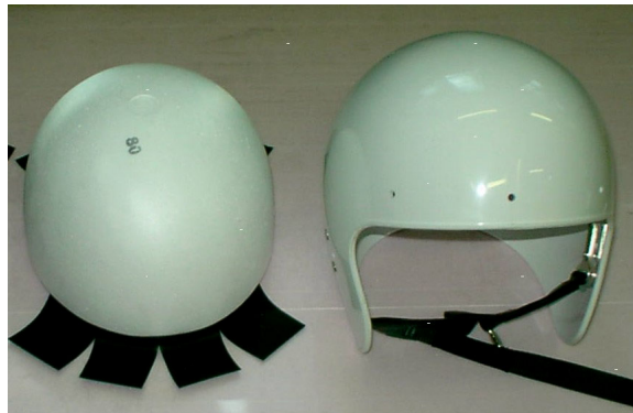
Figure 1 Left: The liner with the protruding black rubber strips. Right: The shell front, to which the rubber strips are taped.
